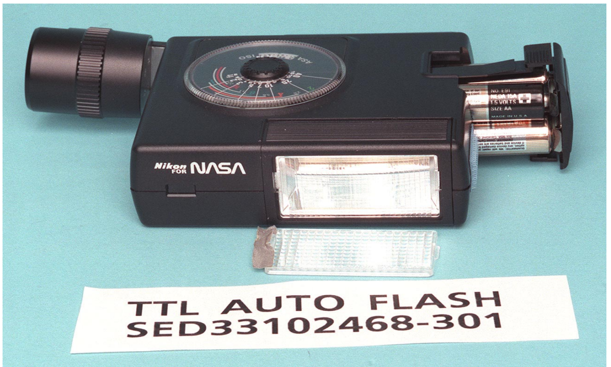
Figure OPS-122 TTL Auto Flash Showing Battery Location with the Flash Diffuser Lens Removed S87-30377
