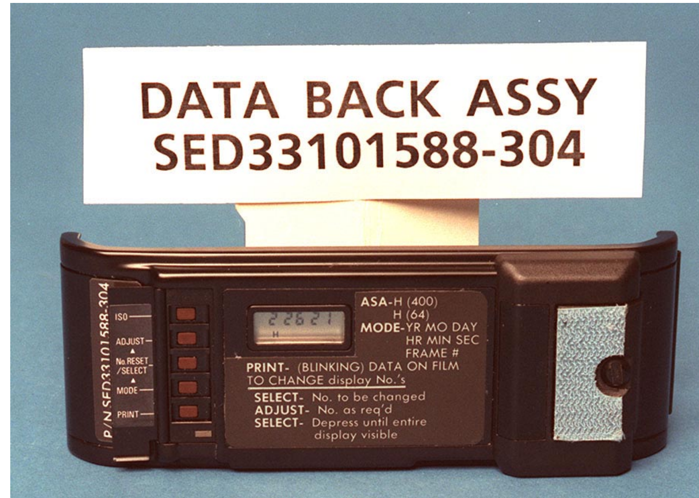
Figure OPS-120 Data Back for F3 Nikon System (Installed Preflight on Camera Back)
