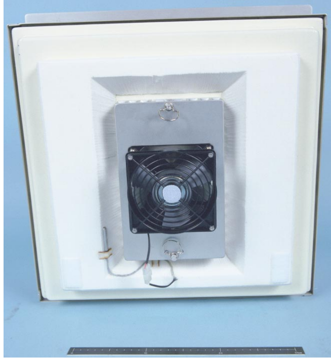
Figure OPS-159 TEHOF Active Lid Interior S97-15730
