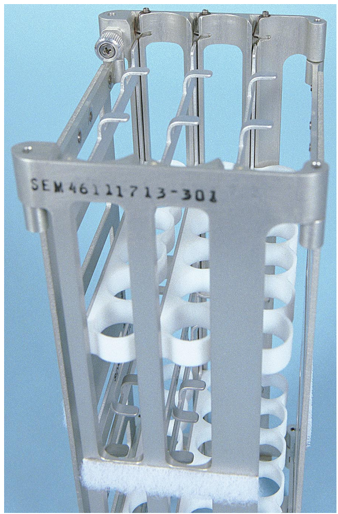
Figure OPS-180 Sample Holder Cage Showing Latches to Secure Sample Cards in Place
