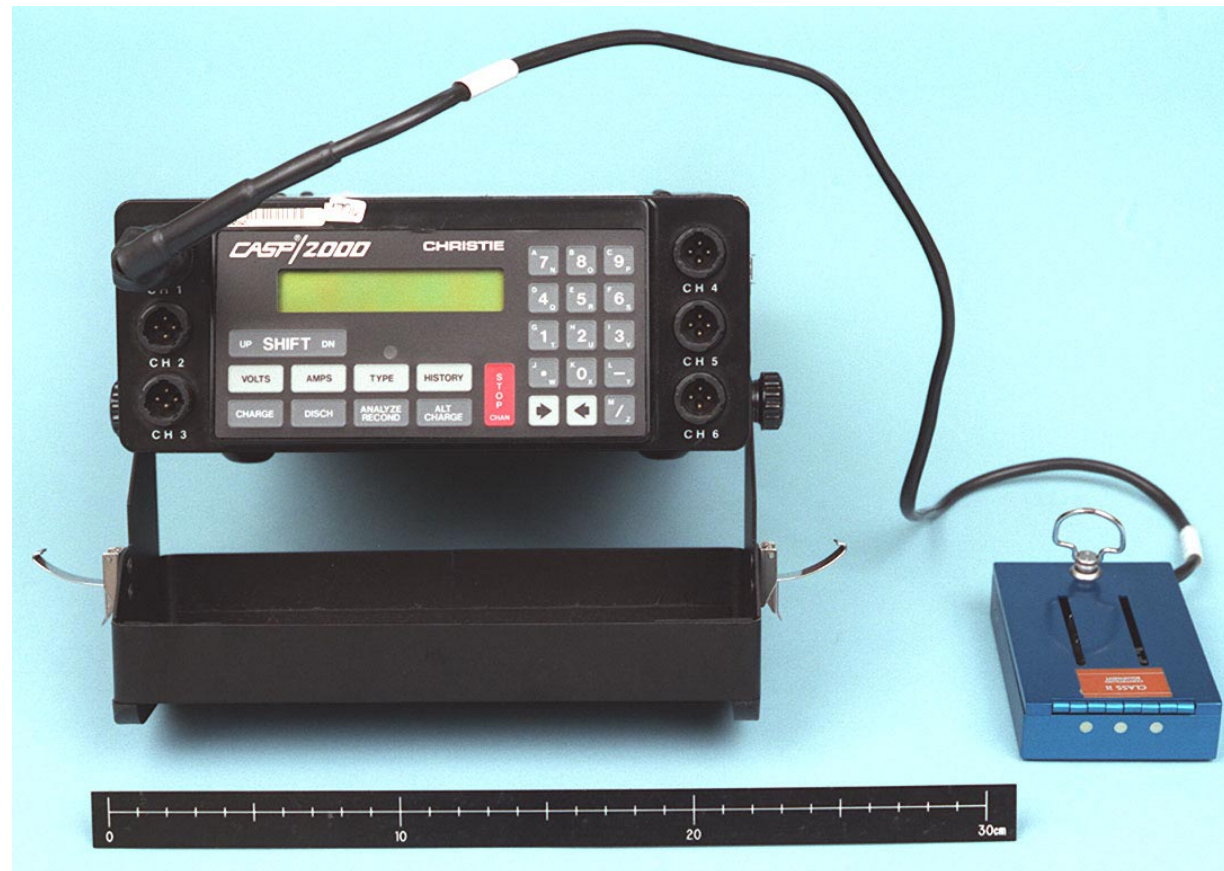
Figure OPS-225 Universal Battery Charger (Flight Version is Without the Stand) Attached to AA Recharge Box
