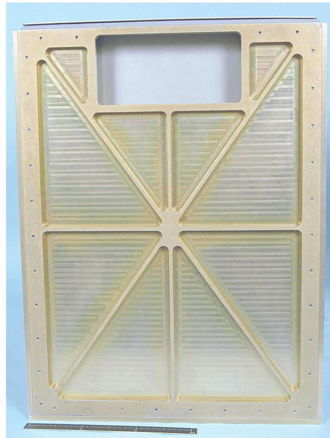
Figure OPS-171 TEHOF Shell Assembly, Side Plate (2 pc); Hole is to Facilitate Air Flow
